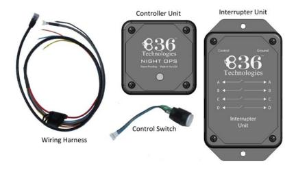
**The Controller Unit** is the heart of the system. It contains a microcontroller which handles all system automation. This unit needs to be mounted on the vehicle dashboard where it will have an unimpeded view of the ambient daylight. A female CAT5 type modular port allows for a quick connection to the wire harness.
